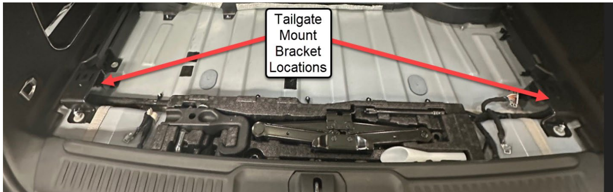
Figure 37-Jeep Wagoneer Tailgate Bracket Location.
