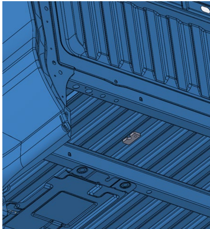
Figure 7-Example of Pleat Spacer Install Under the Truck Box
