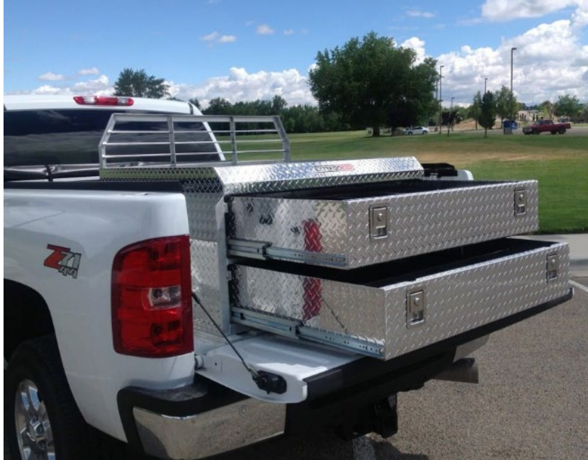
Figure 52-Example of Aluminum Slide Out.
