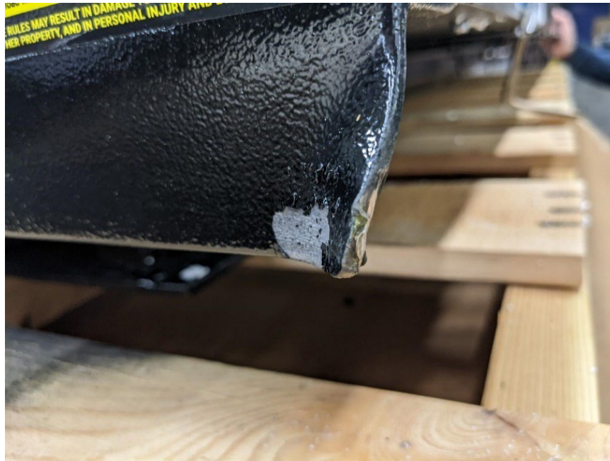
Figure 3-Example of Damage, Bent Corner
